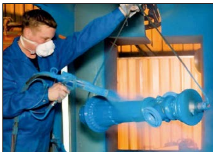
Fig. 7.2.1-04: Electrostatic application of epoxy powder with a spray gun
