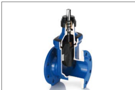
Fig. 7.4.1-02: Sectional image of a resilient seated flanged gate valve with a non-bolted connection between bonnet and body
