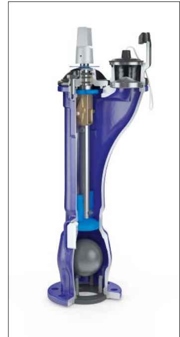
Fig. 7.8.4-02: DN 80 underground hydrant – double shut-off, opening against the direction of flow – fully enamelled
