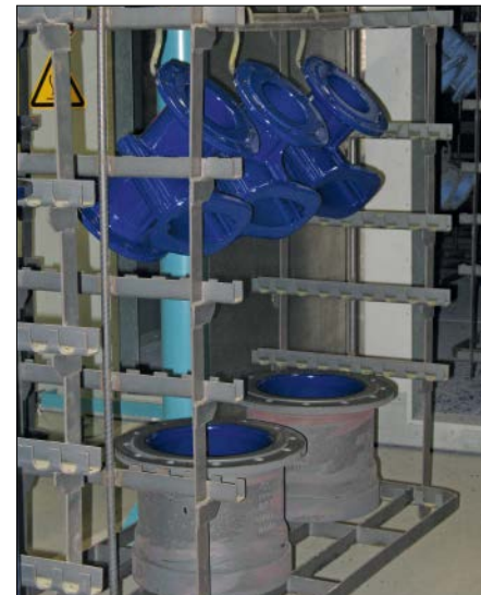
Fig. 7.2.2-07: Enamelled gate valve bodies and fittings after curing
