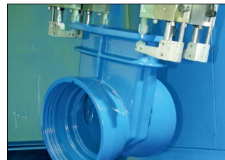
Fig. 7.2.1-07: Gate valve body coated in the fluidised bed of powder
