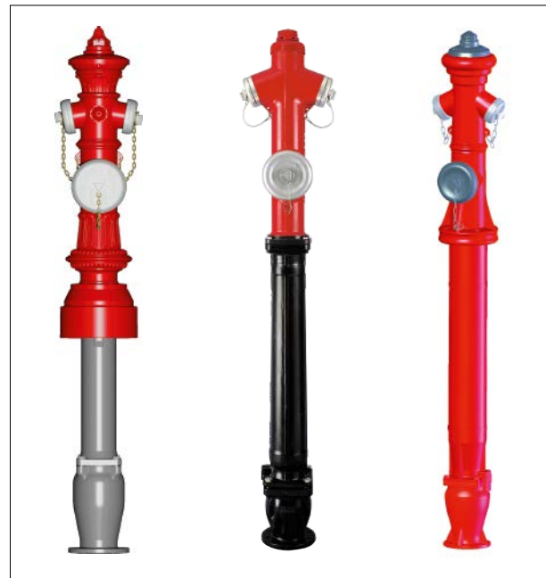
Fig. 7.8.3-02: Design examples – DN 100 pillar hydrant – 2 B outlets, 1 A outlet with flanged joint
