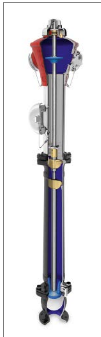
Fig. 7.8.3-06: Cross-section of a DN 100 pillar hydrant with 2 B outlets and 1 A outlet with stainless steel column
