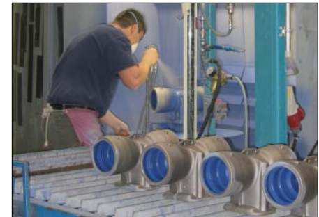
Fig. 7.2.2-04: Slip application on the outside of gate valve bodies by spraying
