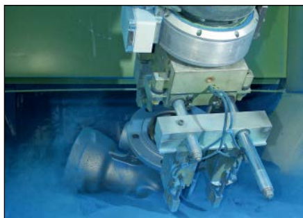
Fig. 7.2.1-06: Dipping a valve body into the fluidised bed of powder
