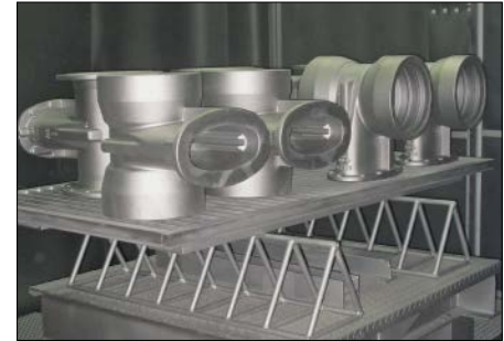
Fig. 7.2.2-03: Gate valve body after blasting
