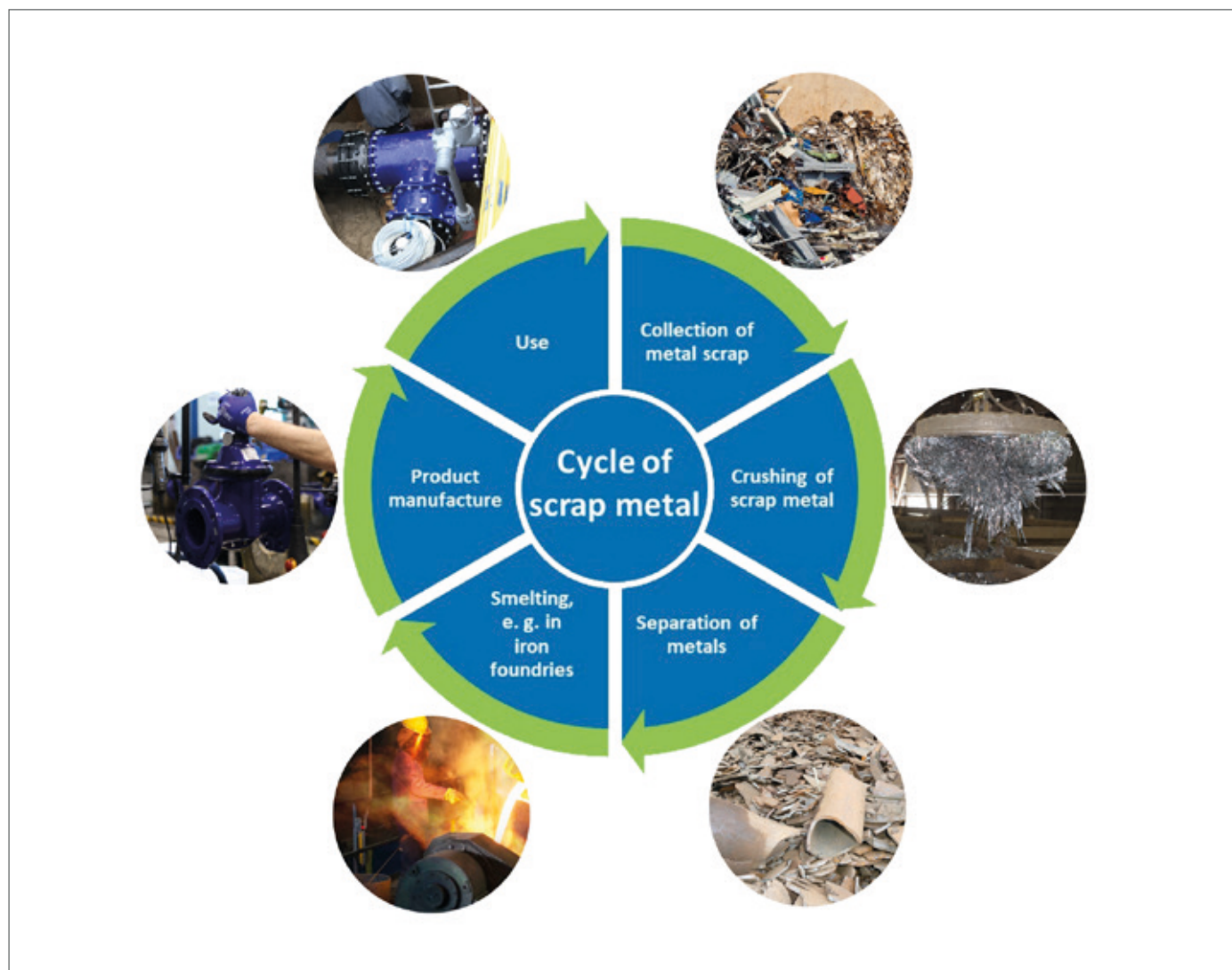
A closed-loop recycling system has already been in operation for the production of cast iron in Europe for many years.
