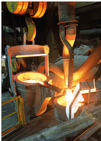
Recirculation of flushing iron with additional ladles and enhanced plant technology. Left: Filling a ladle. Centre: Transport of the still liquid flushing iron to the forehearth. Right: Back into the forehearth and use in the production process.
