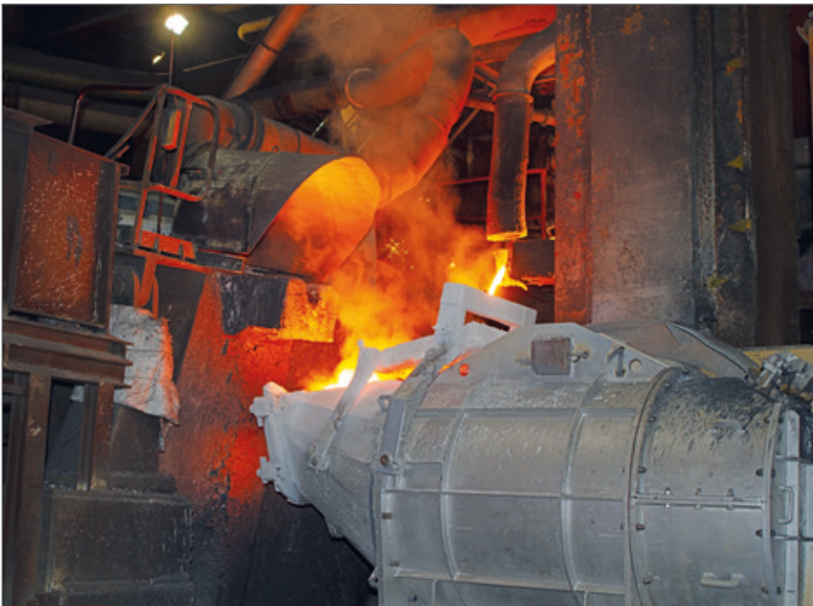
Converter in the area of the forehearth.
