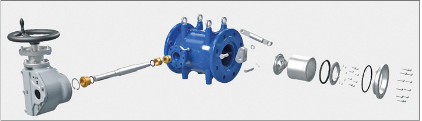
Exploded view of the type 7015 plunger valve: body in spheroidal graphite cast iron; control cylinder and slider-crank mechanism in high-grade steel, steel bolts and brass cylinder liner.
