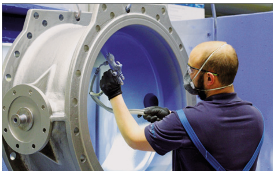
Enamelling for outstanding and long-lasting corrosion protection.
