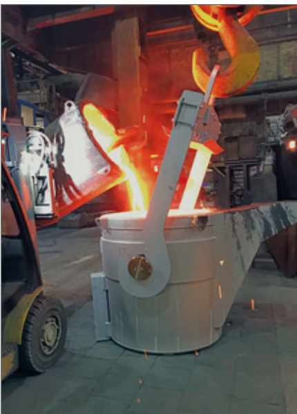
Recirculation of flushing iron with additional ladles and enhanced plant technology. Left: Filling a ladle. Centre: Transport of the still liquid flushing iron to the forehearth. Right: Back into the forehearth and use in the production process.
