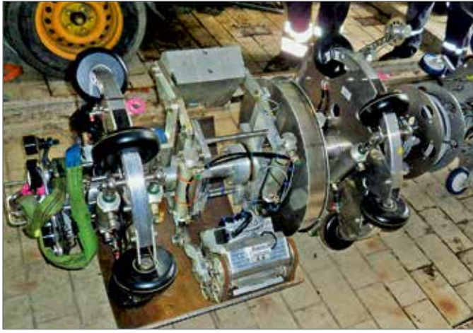
The PLS type SLOFEC® internal pipe scanner.
