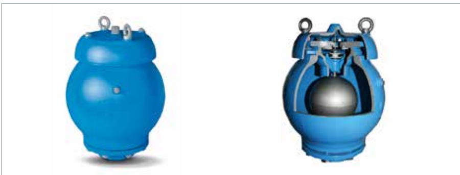
Different construction forms of aeration and air release valves with lever function. Top left: sectional view of a single-chamber valve with valve lever for small and large volumes of air; bottom left: aeration and air release valve with lever function for wastewater pressure pipelines; right: The illustration shows operational air release. The float is attached to a lever. A valve tappet on the lever closes the air release port under positive pressure. With negative pressure, the float drops and the port is opened. Air can escape.
