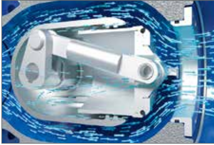
Hygiene safety by systematic flushing of the plunger.
