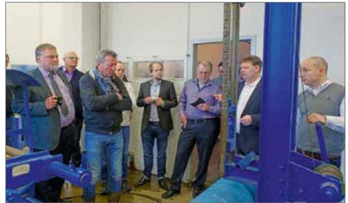
Demonstrating the drop test for checking the impact resistance of cement mortar coatings.
