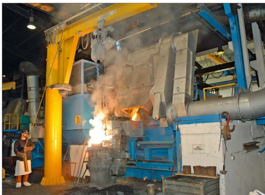
Five-tonne medium frequency induction furnace (source: Ludwig Frischhut GmbH & Co. KG)
