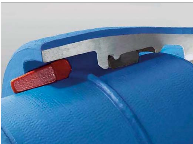
VRS®-T positive locking restrained push-in joint with weld bead, part of the socket opening, locking element (red) and retaining chamber
