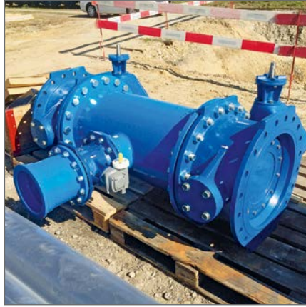
Shut-off unit with vonRoll DN 400/200 butterfly valves, preassembled in the factory
