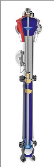
DN 100 pillar hydrant: 2 B outlets and 1 A outlet with stainless steel column
