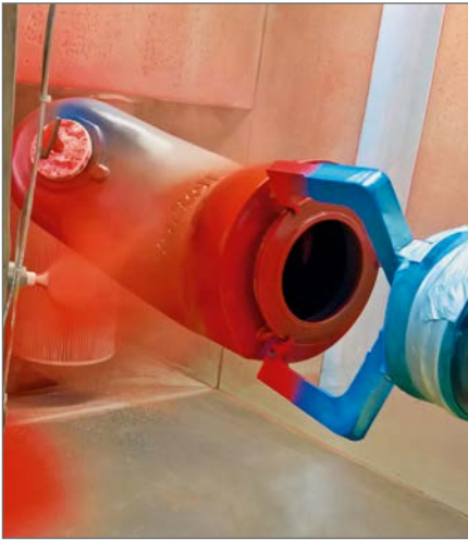
Application of a polyester powder as a surface layer on an epoxy coating by the electrostatic spraying process
