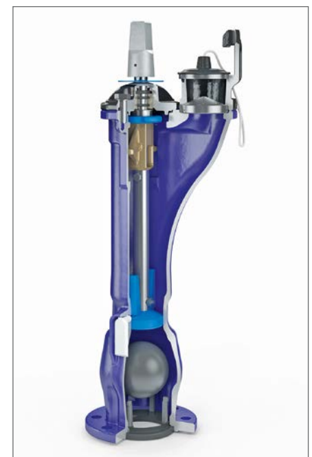
DN 80 underground hydrant: double shut-off, opening against the direction of flow – fully enamelled
