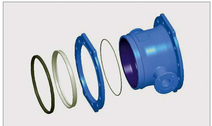
Assembly of the ERHARD ROCO wave loose-flanged butterfly valve: (left to right) sealing ring as flange seal (EPDM), retaining ring (stainless chrome steel 1.4301), loose flange (EKB epoxy coated), O-ring, fixed flange
