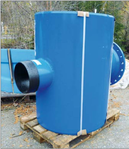
A shaft is installed additional at a low point in the power station pipeline to provide a supplementary flushing facility
