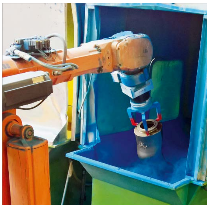
Coating by the fluidised bed process
