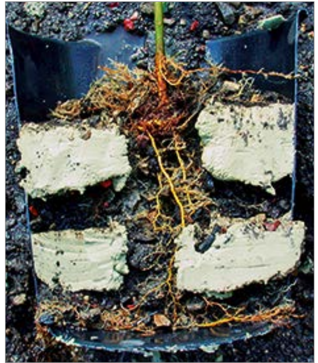
Figure 5: Planter cut open – roots flushed off with water. The roots have not grown into the bentonite. Source: Stützel, T.
