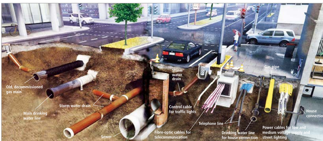
Figure 3: Example of how the underground space beneath a road is used Source: RWE-Magazin June 2006, modified by K. Schröder
