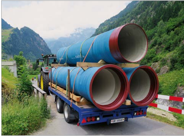
Figure 1: Transporting the DN 1000 ductile iron pipes in the Maderaner valley
