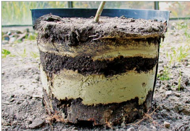
Figure 4: Planter opened down the side – no roots are to be seen in the layers of bentonite Source: Stützel, T.
