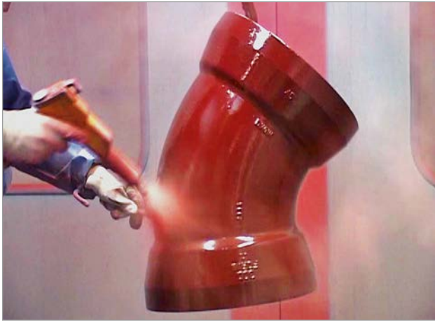
Figure 2: Manual coating process using an electrostatic gun – the powder is melted directly on the hot substrate resulting in the continuous build-up of a film
