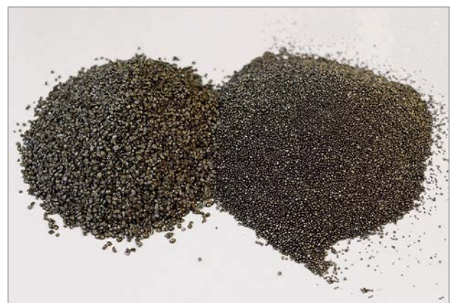
Figure 1: Outwardly recognisable difference of sharp-edged original blasting agent (left) as compared with the “rounded” blasting agent used (right)
