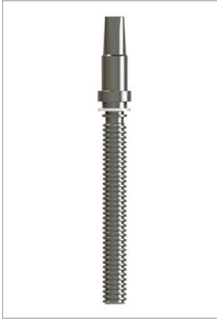
Figure 5: One-piece stem with stem collar – rolled trapezoidal thread
