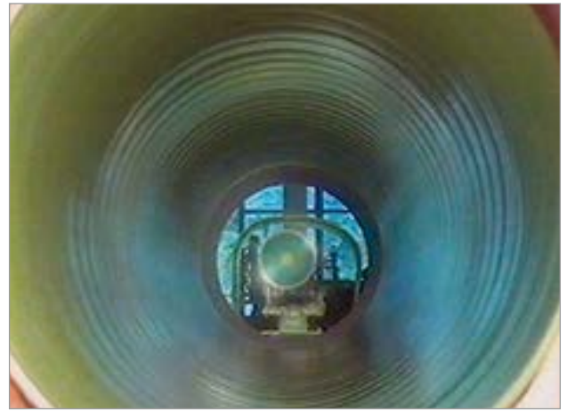
Figure 4: Glassy PUR lining, hydraulically smooth with roughness k \leq 0,01 mm
