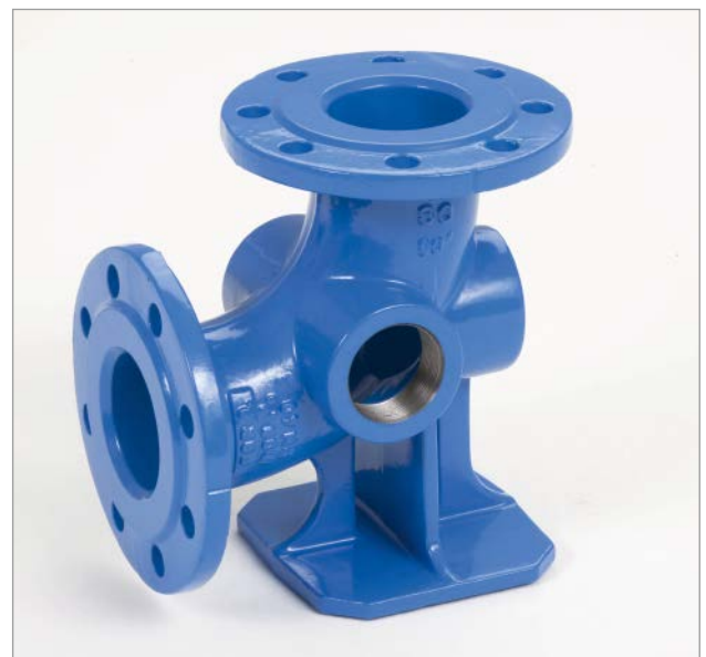
Figure 2: Epoxy powder coated DN 80 double flanged 90° duckfoot bend with PN 40 flanges and three branch connections each with 2" internal thread
