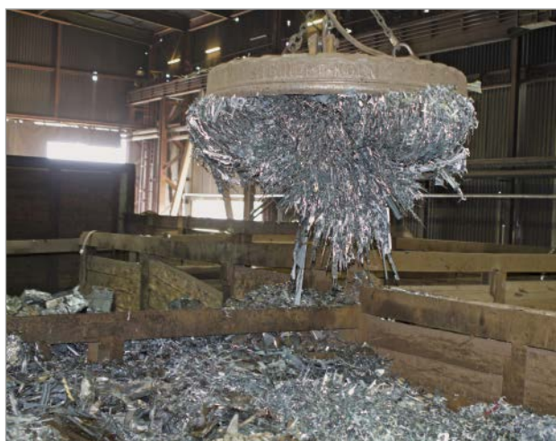
Figure 7: Use of steel scrap for the production of ductile cast iron
