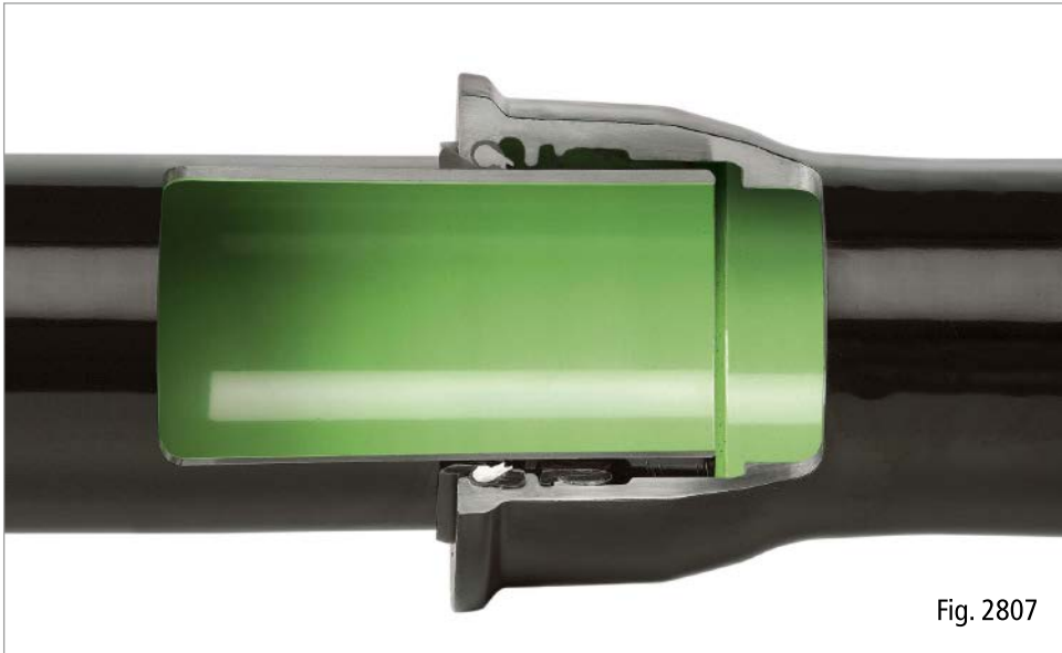
Figure 9: Internal vonRoll HYDROTIGHT thrust resistance system with high electrical resistance for reducing longitudinal electrical conductivity
