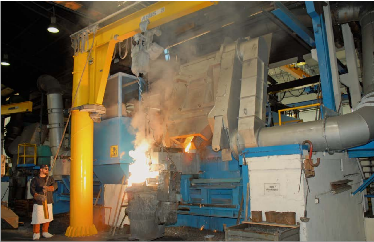
Figure 3: Ultra-modern five tonne medium frequency furnace
