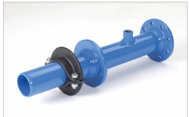
Figure 1: DN 80 flanged spigot coated with epoxy powder in special length L = 800 mm with PN 16 flange and a welded blue, or optional clamp-on black, puddle flange. The flanged spigot is fitted with a branch connection with a 1" internal thread.
