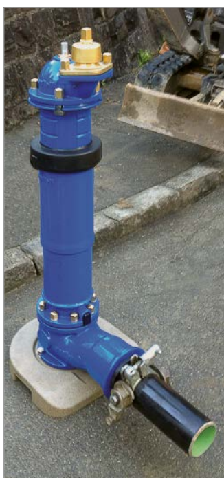
Figure 4: Preparation before installation: optimum stability on the new polymer concrete base – preassembled connection pipe and cover for the design as an underground hydrant
