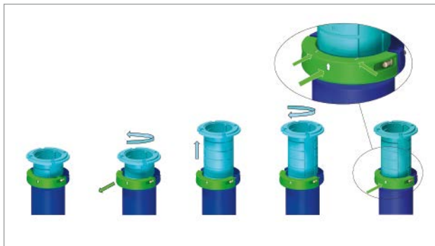
Figure 3: Extremely simple height adjustment with the patented bayonet system
