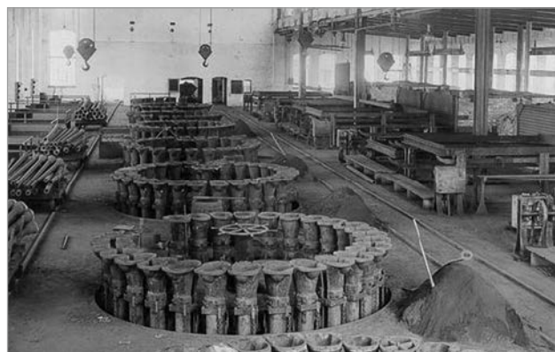
Figure 2: Production of cast iron pipes with casting carousels (around 1900)
