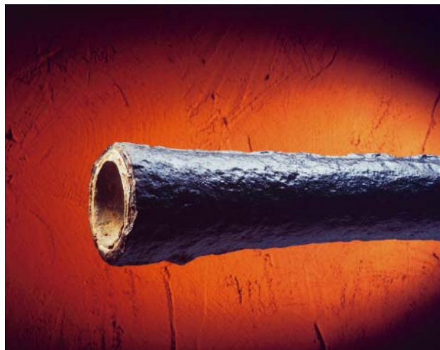
Fig. 7: Cast iron pipe, as was installed in Dillenburg Castle until 1760
