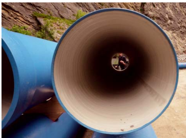
Fig. 7: DN 800 ductile iron pipes with cement mortar lining
