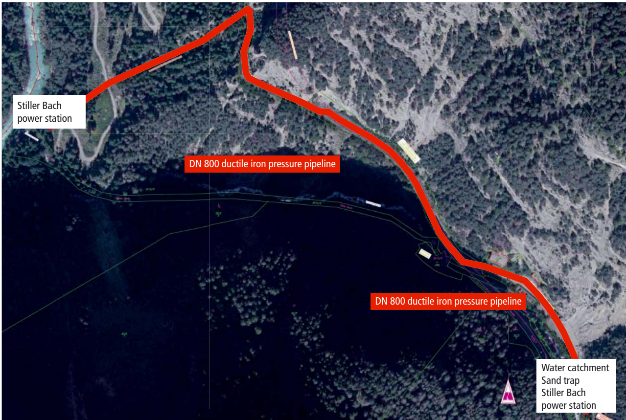
Fig. 2: The route of the DN 800 pressure pipeline for the Stiller Bach power station
