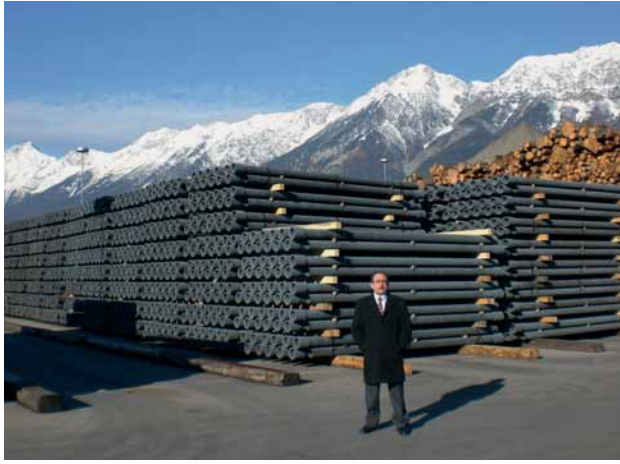
Fig. 3: 5 m long driven ductile iron piles stored ready for delivery
