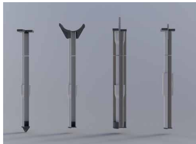
Fig. 10: Types of driven ductile iron piles – tension and compression piles: depending on the nature of the soil and the loads, ductile iron piles with suitable top and bottom accessories are installed with or without grouting.
