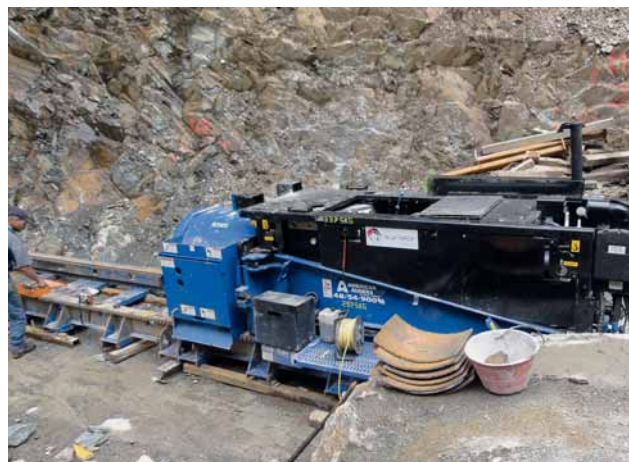
Fig. 7: The diesel-hydraulic traction unit at the tunnel exit. It was also converted to act as the boring unit
