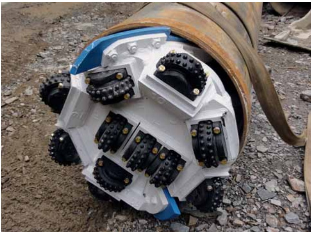
Fig. 4: DN 800 boring head, showing replaced cutting wheels
