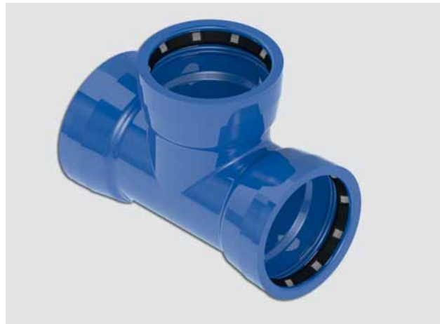
Fig. 3: All-socket tee with 90° branch for drinking water, TYTON® socket with inset TYTON SIT PLUS® gasket (EPDM)
