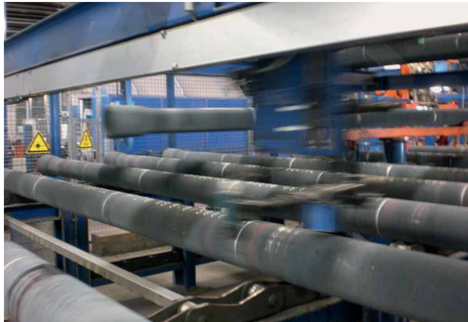
Fig. 2: Driven ductile iron piles are preformed industrially under very strict quality controls during the process. Together with the barrel of the pile pipe, the conical plug-in joint is produced in a single cast.
