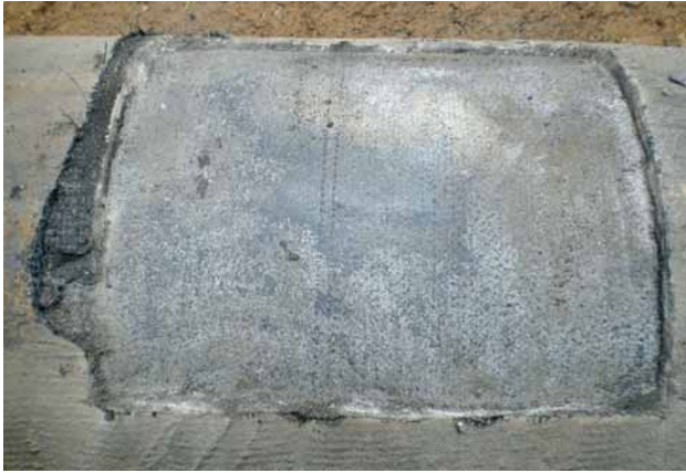
Fig. 2: Project 1: DN 400 ductile iron pipe - ZM-U with epoxy bonding layer and zinc coating; no visible signs of corrosive attack
