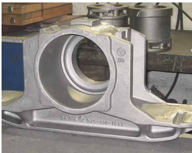
Fig. 8: A railway axle box of EN-GJS-400-18-LT ductile iron
