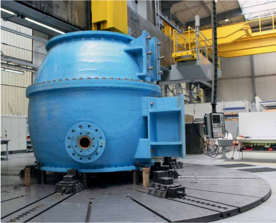
Fig. 4: The inner circumference of the valve being machined on a vertical turret lathe
