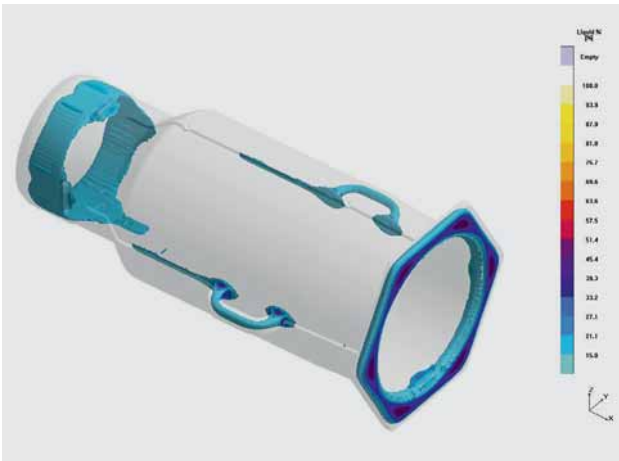
Fig. 2: Solidification 1, molten metal and the slowly increasing parts of it which are solid, shortly before complete solidification (everything in see-through form)
