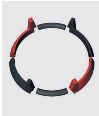
Fig. 7 (on the left): The BLS® push-in joint
