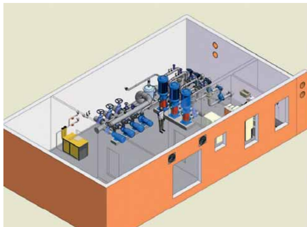
Fig. 5: The main pumping station
