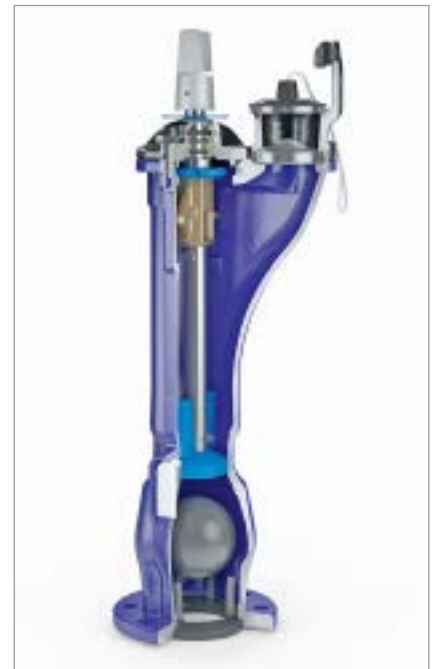
DN 80 underground hydrant: double shut-off, opening against the direction of flow – fully enamelled
