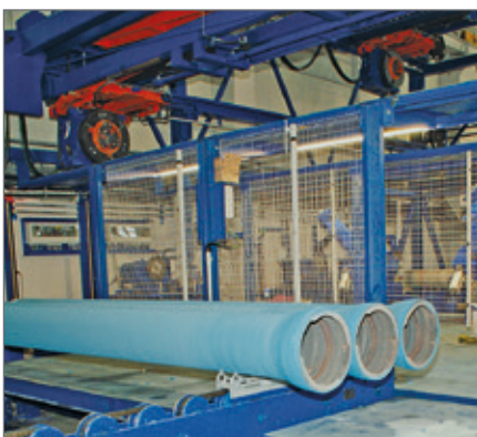
The roughness of the galvanised outside surface helps the new type of cement mortar to adhere to the pipe in the best way possible.
