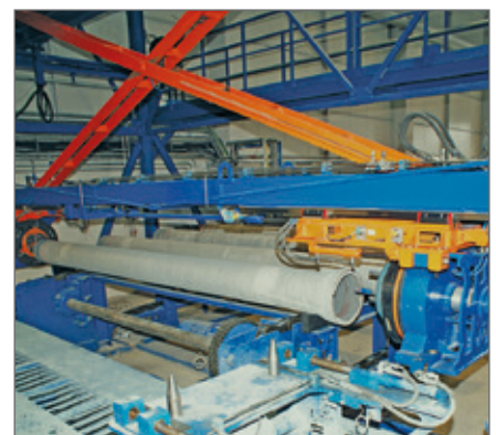
Two wrapping machines which, in recent weeks, have been optimally adapted to the production processes, are capable of coating pipes from DN 80 to DN 1000.
