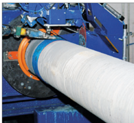
The fibre cement coating is applied in a thickness of 5 mm in a fully automatic extrusion process.
