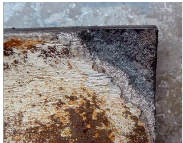
Figure 3: Section of cast iron pipe with partially removed cement mortar lining
