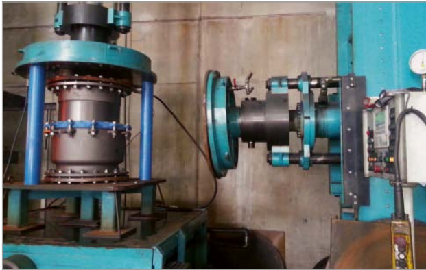
Figure 5: Function testing with E-Flex and spigot end with extreme dimensions
