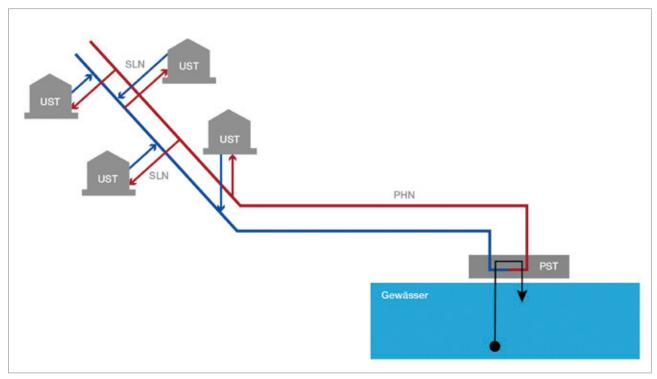
Diagram showing an example of an Anergy network.
