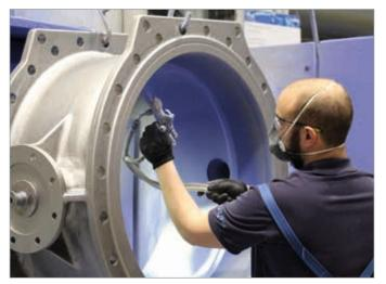
Application of the enamel coating by spraying
