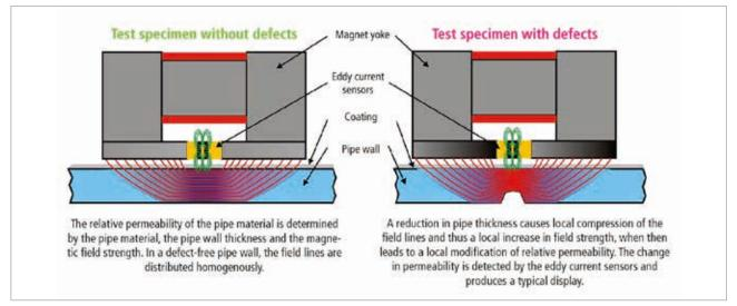
SLOFEC<sup>™</sup> functioning principle
