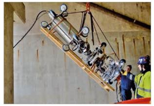
Lowering the SLOFEC<sup>®</sup> scanner into the lower head of the culvert
