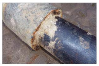
The PLUG & DRIVE<sup>®</sup> joint of a cast iron driven pile extracted after 30 years
