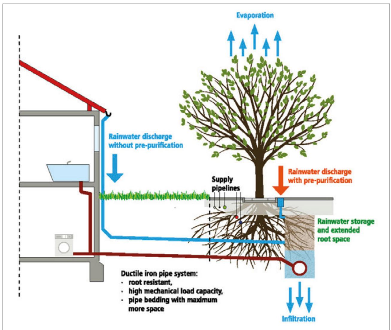
The sponge city principle in the street space. By the use of large-grain, broken materials with a large storage volume, the soil in the pipeline trench becomes a rainwater storage space and provides extended root space.
