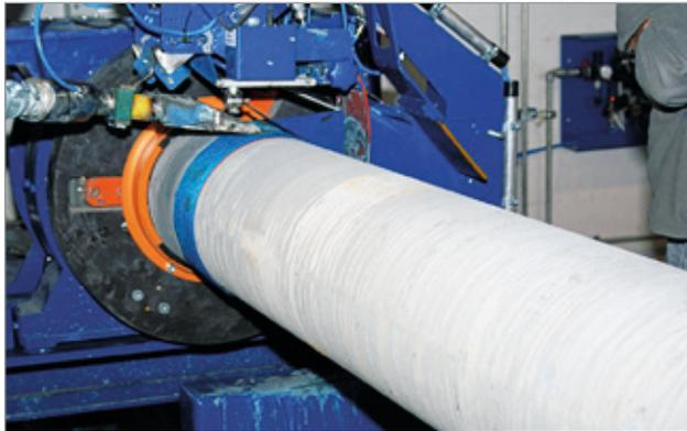
The fibre cement coating is applied in a thickness of 5 mm in a fully automatic extrusion process.
