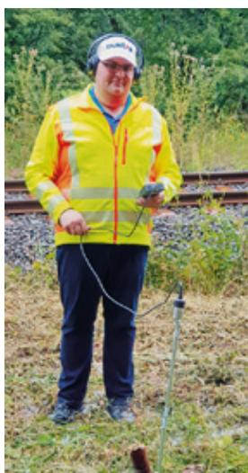
On-the-spot confirmation of measurement results with a ground microphone.
