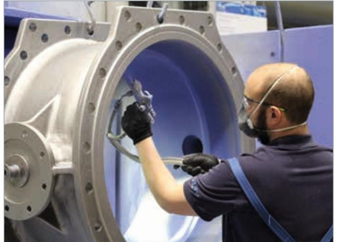
Application of the enamel coating by spraying
