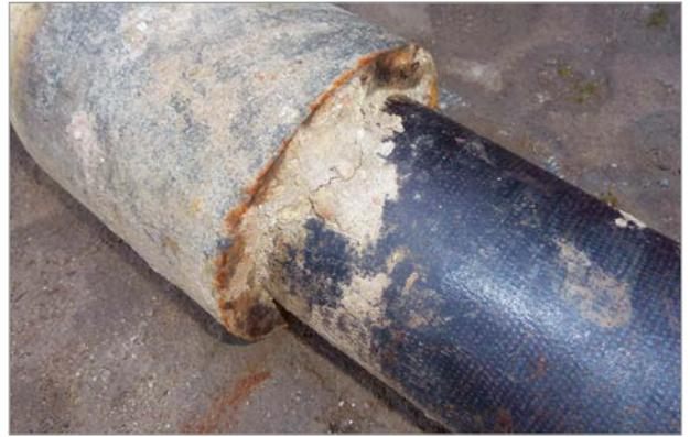
The PLUG & DRIVE® joint of a cast iron driven pile extracted after 30 years
