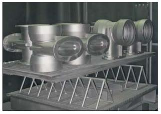
**Fig. 7.2.2-03:** Gate valve body after blasting
