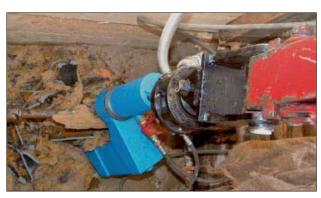
**Figure 22.18:** Hydraulic pipe cracker
