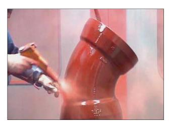
**Fig. 3.30:** Electrostatic application of epoxy powder with a spray gun
