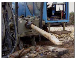
**Figure 22.24:** Drill head for pilot boring
