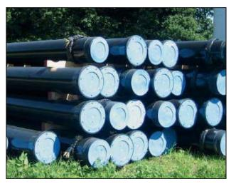
**Fig. 14.5:** Ductile iron pipes with a polyethylene coating
