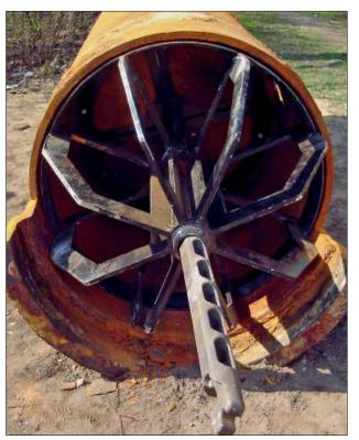
**Figure 22.50:** Tool for removing incrustations
