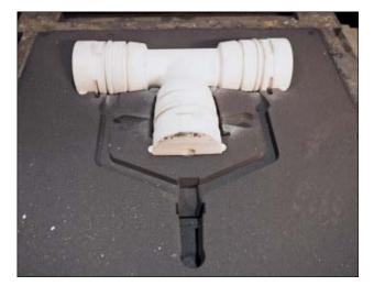
Fig. 3.18: Lost core inserted in the sand mould
