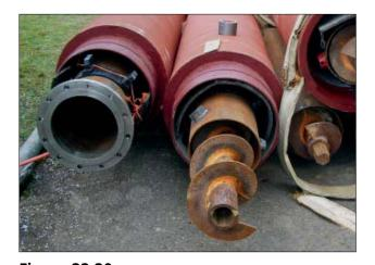
**Figure 22.20:** ZM-U-Plus cement mortar coated sewage pipe fitted with feed tube and string of auger sections
