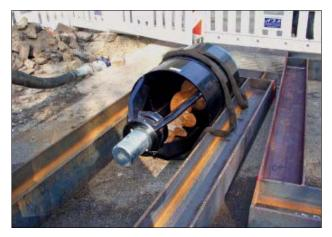
**Figure 22.19:** Traction head with internal feed auger
