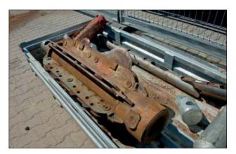
**Figure 22.13:** Cutting whell for old pipes in steel
