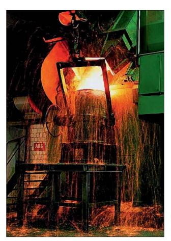
**Fig. 3.4:** Electrical induction furnace
