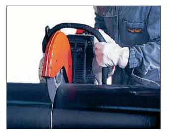
**Fig. 19.17:** Separation cut on a pipe
