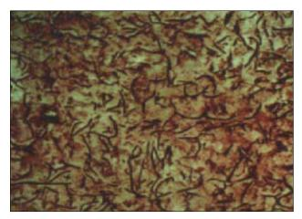
**Fig. 2.1:** Cast iron with lamellar graphite (grey cast iron)
