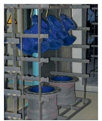
**Fig. 7.2.2-07:** Enamelled gate valve bodies and fittings after curing
