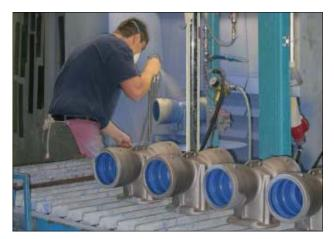
**Fig. 7.2.2-04:** Slip application on the outside of gate valve bodies by spraying
