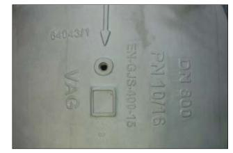
**Fig. 3.39:** Marking of a plunger valve, DN 800, PN 10/16
