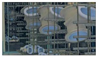
**Fig. 7.2.2-05:** Internally coated gate valve bodies in the drying line
