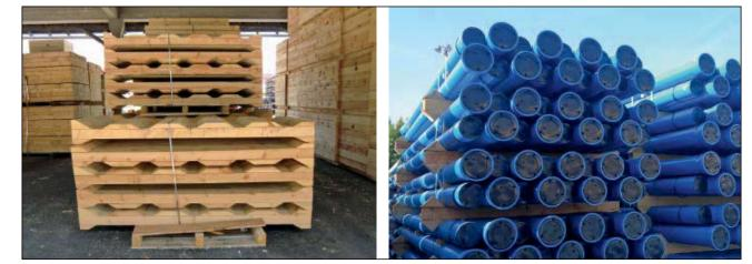
**Fig. 19.6:** Ductile iron pipes stacked with the help of wooden supports
