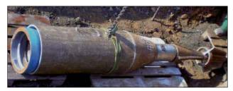
**Figure 22.7:** Bursting head with ribs, upsizing element and traction head
