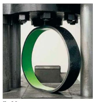
**Fig. 2.8:** Ring flattening test
