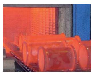
**Fig. 15.6:** Fittings during the enamel firing
