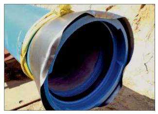
**Figure 22.46:** Sheet steel cone for protecting the socket
