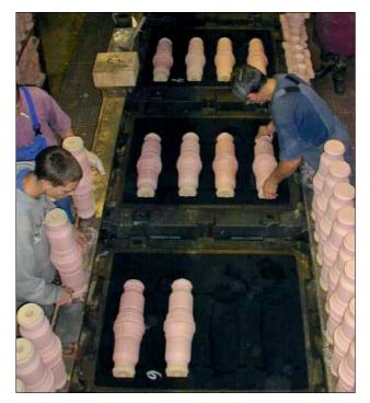
**Fig. 3.15:** Production of fittings with lost cores
