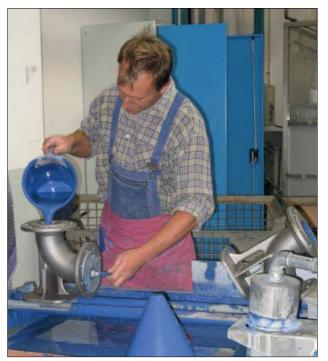
**Fig. 3.32:** Applying enamel by pouring
