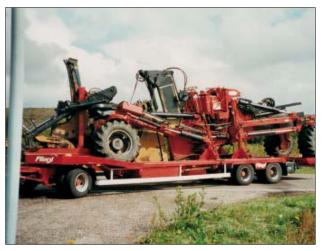
**Figure 22.36:** Plough The plough is attached by a steel cable **(Figure 22.37)** to the towing vehicle, which can be supported by a plate on the ground to transmit the traction forces into ground.
