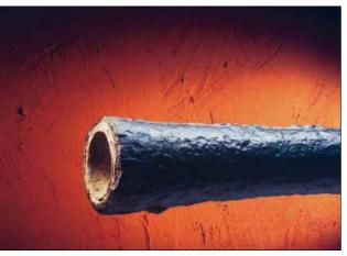
**Fig. 1.1 :** Cast iron pipe from the water supply pipeline for Dillenburg Castle (1455)
