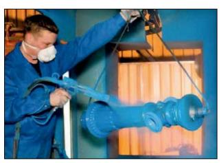
**Fig. 7.2.1-04:** Electrostatic application of epoxy powder with a spray gun
