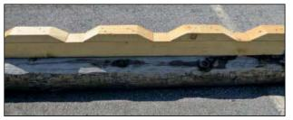
**Fig. 19.3:** Sleeper for stacking ductile iron pipes
