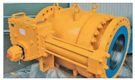
**Fig. 7.6.18:** Pilot-operated plunger valve driven by its own medium
