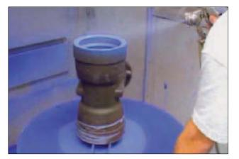
**Fig. 3.33:** Applying enamel by spraying
