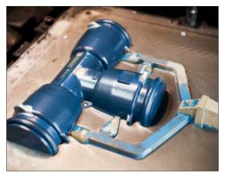
**Fig. 3.16:** Pattern for the production of the sand mould
