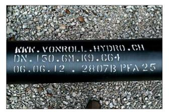
**Fig. 3.35:** Marking of a ductile iron pipe with restrained flexible push-in joint in accordance with [3.16]
