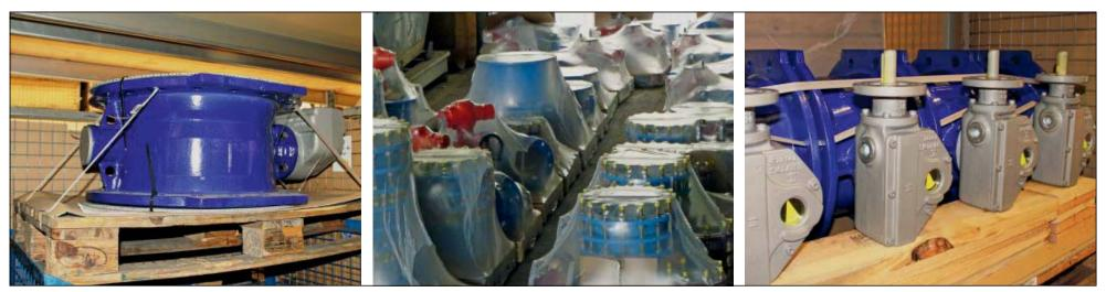
**Fig. 19.13:** Arrangement of valves on disposable pallets ready for dispatch
