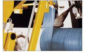
**Fig. 3.24:** Cement mortar coating – extrusion process
