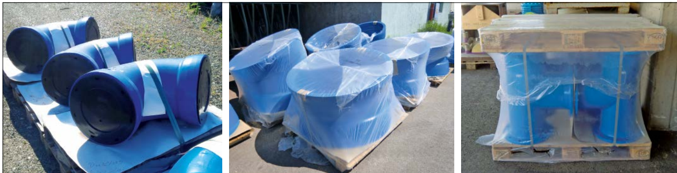
Fig. 19.11: Preparation of fittings ready for dispatch on disposable pallets
