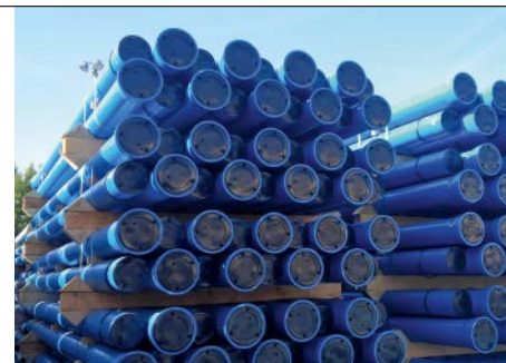
Fig. 19.6: Ductile iron pipes stacked with the help of wooden supports
