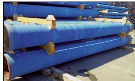
Fig. 19.15: Ductile iron pipes > DN 300 suitable for cutting on site – marked with a longitudinal white stripe
