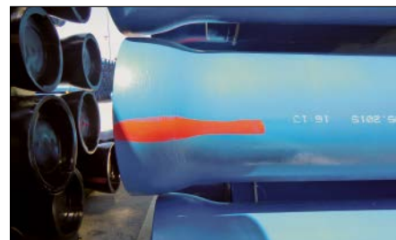
Fig. 19.16: Cutttable ductile iron pipes > DN 300 – marked with a red stripe on the socket – cutting of the pipes from the spigot end to up to 1 m before the socket end-face
