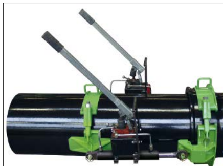
Fig. 19.22: Example of assembly equipment for pulling ductile iron pipes \geq DN 350 together
