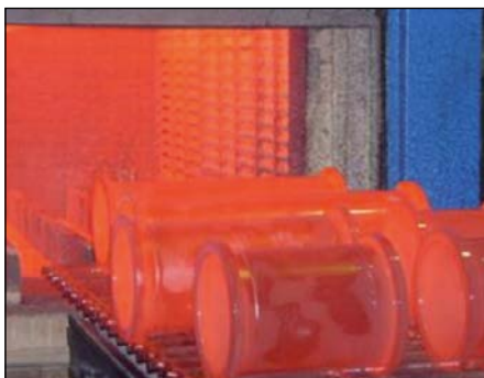
Fig. 15.6: Fittings during the enamel firing
