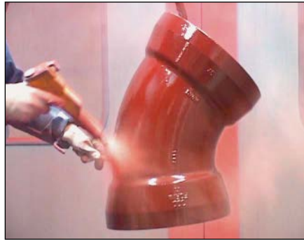
Fig. 15.4: Electrostatic application of epoxy powder by means of a spray gun
