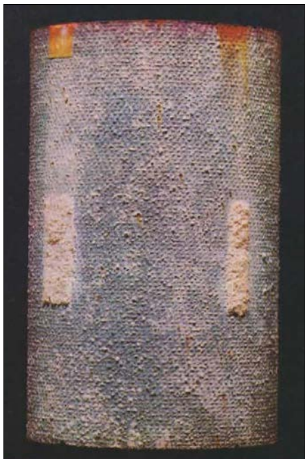
Fig. 14.1: Autogenous healing of artificial injuries by products of reaction of zinc
