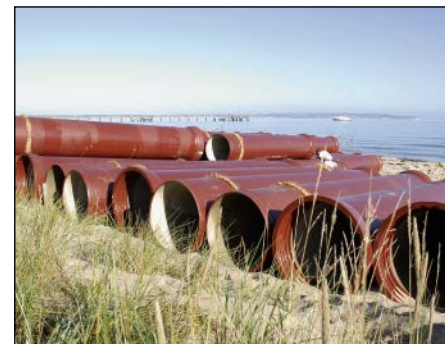
Fig. 14.3: Ductile iron sewer pipes to EN 598 [14.2] with a zinc coating and a reddish-brown coloured finishing layer of bituminous paint.
