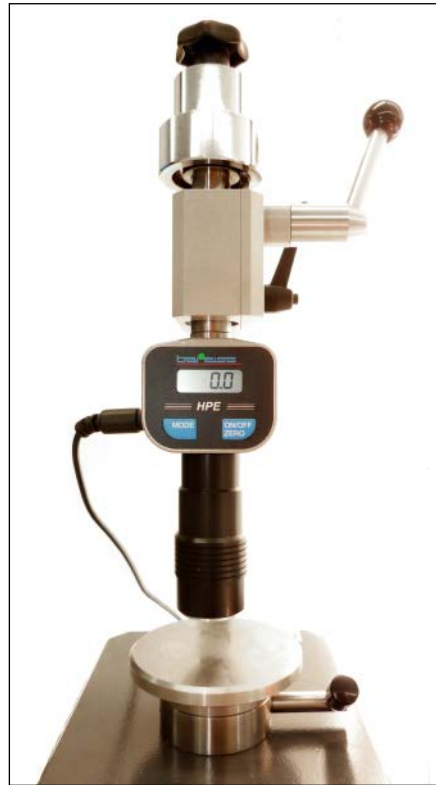
Fig. 13.6: Durometer for measuring rubber hardness according to Shore-A
