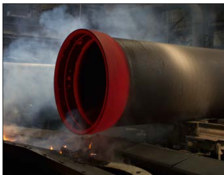
Fig. 3.9: Iron pipe is pulled out of the casting machine socket-end first
