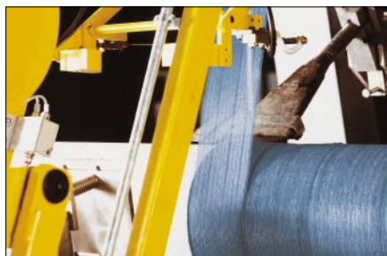
Fig. 3.24: Cement mortar coating – extrusion process
