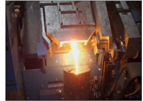
Fig. 3.3: Discharge of molten iron from the mixer
