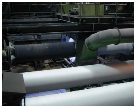
Fig. 3.21: Applying the zinc-aluminium coating
