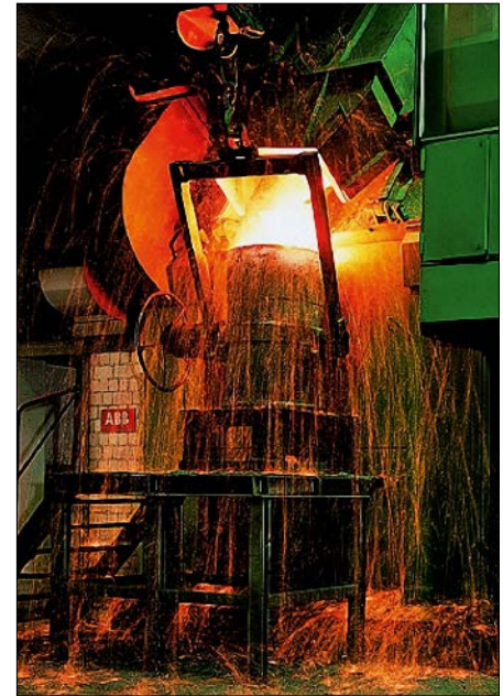
Fig. 3.4: Electrical induction furnace
