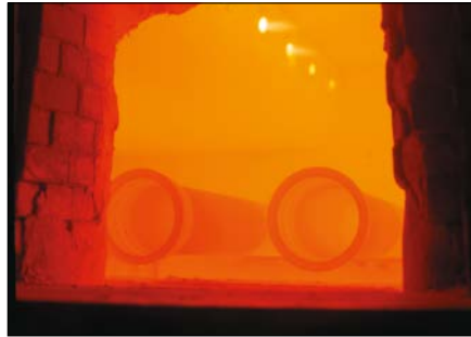
Fig. 19: Pipes in the continuous annealing furnace
