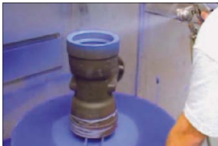
Fig. 3.33: Applying enamel by spraying
