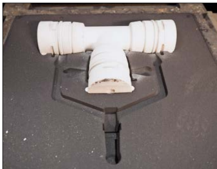
Fig. 3.18: Lost core inserted in the sand mould
