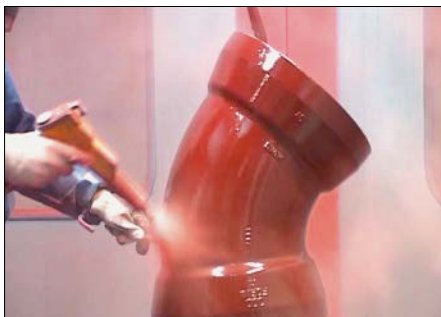
Fig. 3.30: Electrostatic application of epoxy powder with a spray gun
