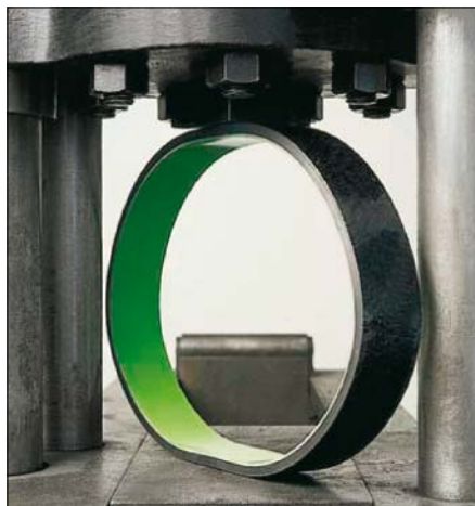
Fig. 2.8: Ring flattening test
