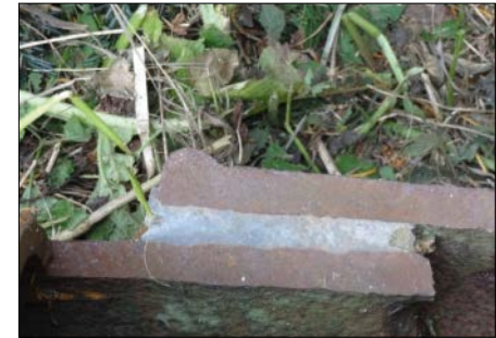
Fig. 1.6: Cut section of a packed socket joint from an approximately 300 year old cast iron pipe – water supply pipeline for the cascades at the Kassel-Wilhelmhöhe castle park with the Hercules monument; UNESCO World Heritage site since June 2013 Source: mhk, Museumslandschaft Hessen Kassel
